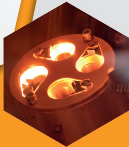
Co-evaporation of up to 4 materials
